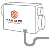
9 VERIFY WALL OUTLET IS CORRECT VOLTAGE AND AMPERAGE. DOES REQUIRE A DEDICATED 120V 15 AMP CIRCUIT.
